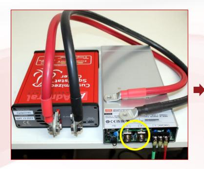
The power supply features V+ and Vterminals to connect to the Cycler, as shown circled in yellow above.
