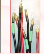
The terminal block has three 10 AWG wires per the number of BIC-2200 power supplies in the stack. The wires are color coded as **black AC/N, green ground (**\\equiv **)**, and **red AC/L.** Each wire has a ring terminal to connect to each BIC-2200 in the stack.
