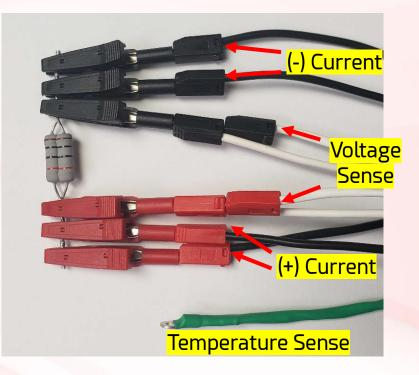
\*The standard 2mm alligator clip shipped with the device is rated for no more than 10A. The standard cable wiring is rated for no more than 6A. Individual current connections per channel are **required** when using the standard cable/alligator clip. A custom cable designed for a single current carrying connection is available for purchase.
