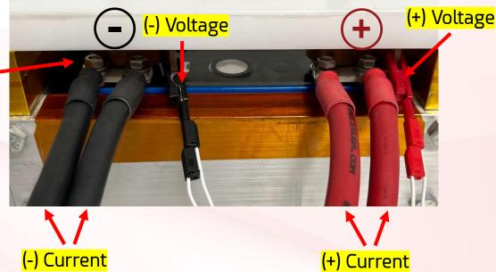
IMPORTANT NOTE: The thick gauge cabling we provide is only rated to carry the amount of current from a single channel. When running in parallel mode, DO NOT attempt to bypass these configuration instructions by running a single current carrying cable from the channel to the device under test. Doing so risks melting the cable.
