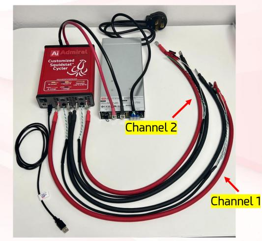
This picture shows how everything should look for a 2-channel configuration above ±10A per channel with a single BIC-2200 at this stage of setup.
