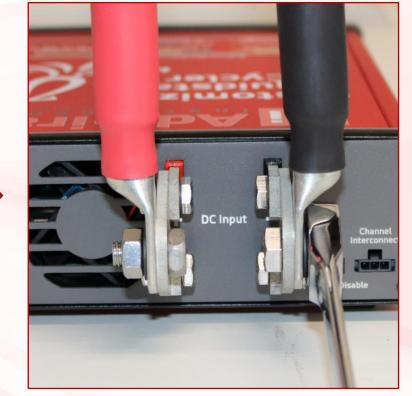
IMPORTANT: All connections must be tightened with wrenches. Loose connections may cause excess heat and risk arcing or fire. DO NOT connect the Squidstat Cycler to the provided power supply yet
