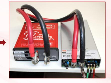
Unscrew any hardware that may be attached to the terminals. Then take the ends of the red/black cables from the Cycler and install them as shown above. V+ is **red** and V- is **black**. IMPORTANT: All connections must be tightened with a screwdriver. Loose connections may cause excess heat and risk arcing or fire. DO NOT connect the power supply to a power source yet.
