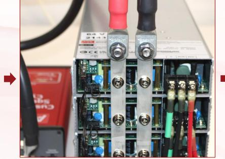
Unscrew any hardware that may be attached to the terminals. Then take the ends of the red/black cables from the Cycler and install them as shown above. V+ is **red** and V- is **black**.
