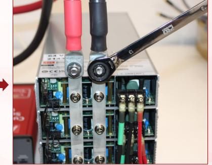
IMPORTANT: All connections must be tightened with a screwdriver. Loose connections may cause excess heat and risk arcing or fire. DO NOT connect the power supply to a power source yet.
