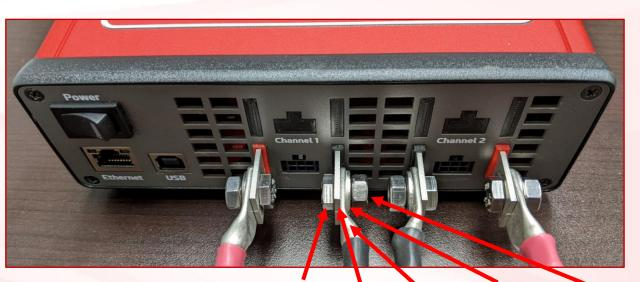
Please <u>precisely</u> match the bolt ↔ tab ↔ lug ↔ washer ↔ nut parts orientation shown in this picture to ensure proper fit and clearance. The bolt heads should be facing the Molex connectors, and the lug/washer/nut combination is on the exterior of the tabs
