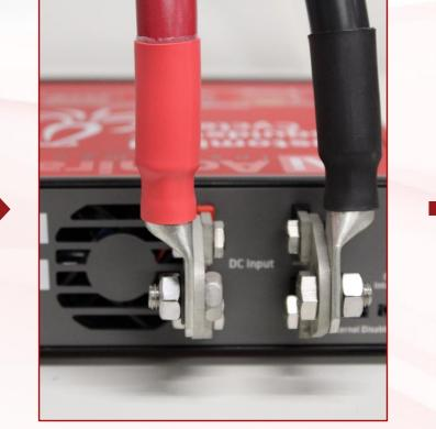
Unscrew the nuts and remove the washers and bolts on both tabs. Then install the red/black cables and reattach the bolt/washer/nut assemblies, as shown above, matching red-to-red and black-to-black.
