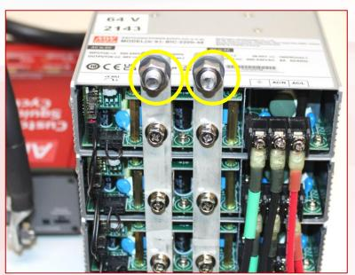
The power supply features V+ and Vterminals to connect to the Cycler, as shown circled in yellow above.
