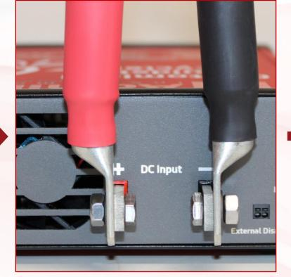
Unscrew the nuts and remove the washers and bolts on both tabs. Then install the red/black cables and reattach the bolt/washer/nut assemblies, as shown above, matching red-to-red and black-to-black.
