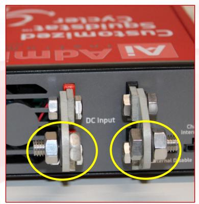
The back of the Squidstat Cycler has two tabs to connect power cables with two sets of M8 bolt/washer/nut assemblies pre-inserted into two joiner plates, as shown above.
